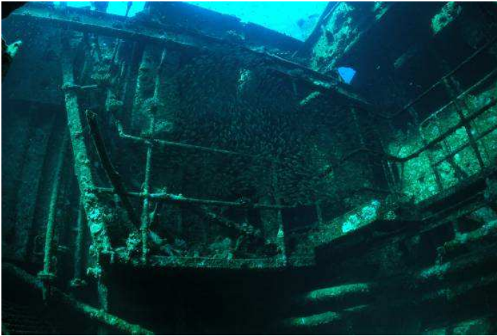
Two views of the engine room house from within. Most of the skylight assembly has now Collapsed,- permitting strong sunlight to penetrate
