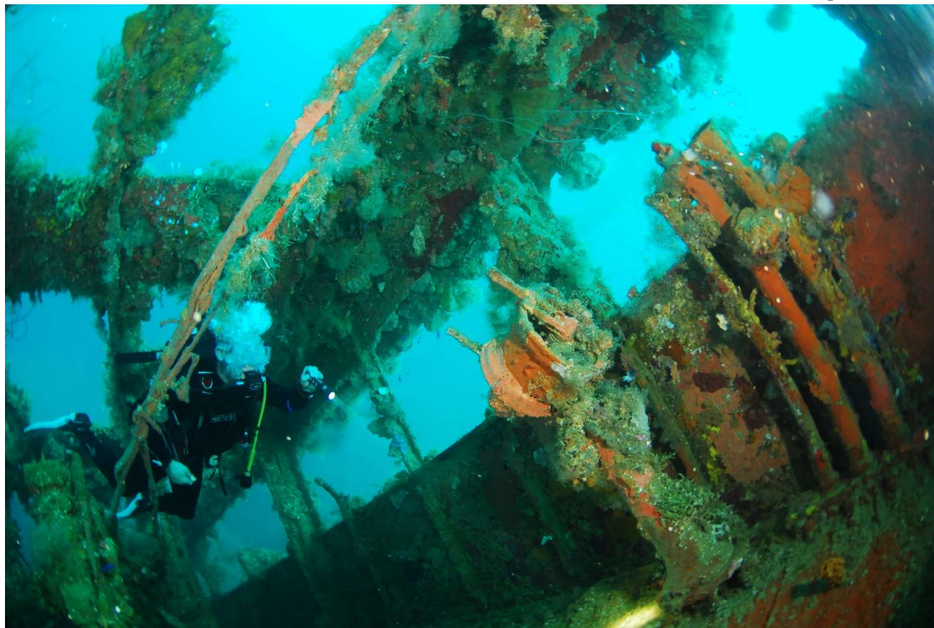
The open bridge/navigation deck sports her instruments to this day; telegraph and voice pipes covered in sea squirts. Bottom left is the rudder stand (helm)
