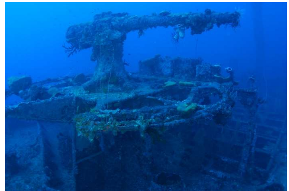
The stern gun, mounted on its pedestal, showing it's framework due to the lack of the wooden floor
