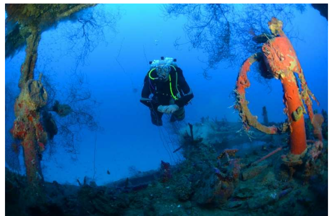
AFT STEERING GEAR WOODEN WHEEL & SPOKES GONE LEAVING ONLY THE BRASS BAND HANGING ON THE RUDDERSTAND
