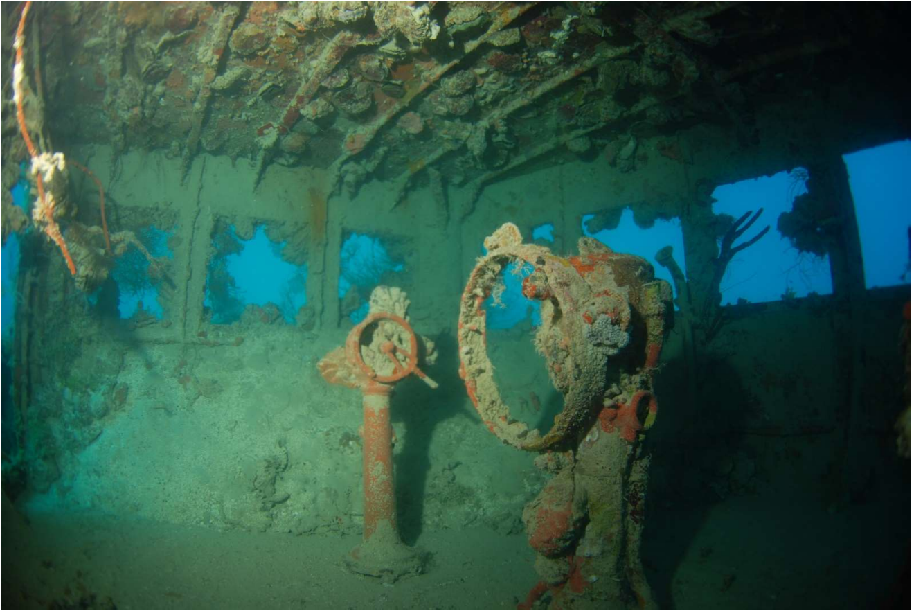
Telegraph, rudderpost, voice pipes-all still in situ in the tugs wheel house.
